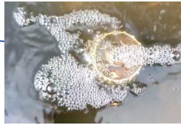
Upper O-Ring leak on underground tank
